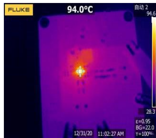
Figure 22. Thermal, 12 VIN, 1 Vout, 5A
